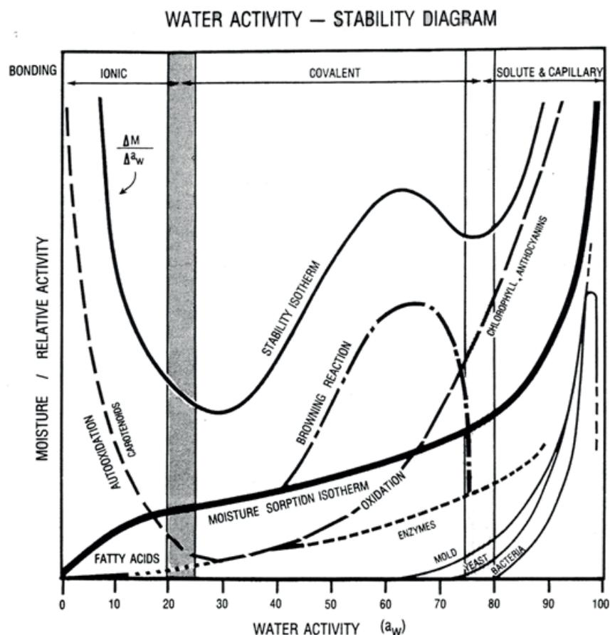
Figure 5. Water activity stability diagram showing the impact of water activity on various degradative reactions that shorten shelf life.
