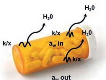
Figure 8. Diagram showing the movement of water in or out of a packaging material as determined by the difference in water activity inside and outside the packaging and the water vapor permeance ( $k/x$ ) of the packaging material.
